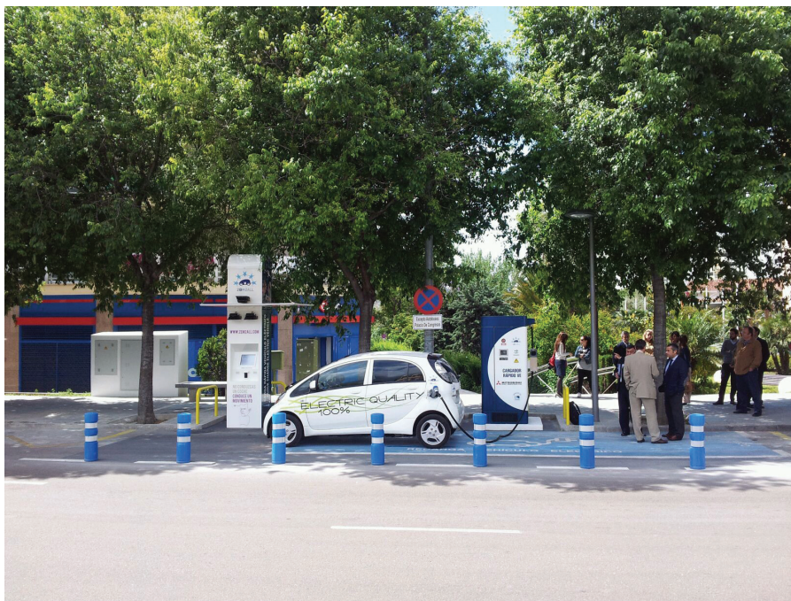
Fig. 3. Mitsubishi Heavy Industries, proiectul ZEM2ALL, Málaga, Spania: Alimentatoare rapide pentru vehicule electrice / Quick charger for electric vehicles Foto / Photo: Mitsubishi Heavy Industries
