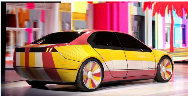
Fig. 15. BMW iVision Dee – Expo CES 2023, Las Vegas – S.U.A. Autovehiculul are 240 de panouri individuale E-Ink, care pot afișa până la 32 de culori diferite, combinațiile acestora fiind nelimitate/ BMW iVision Dee – CES Expo 2023, Las Vegas – USA. The vehicle has 240 individual E-Ink panels, which can display up to 32 different colours and their combinations are unlimited.
